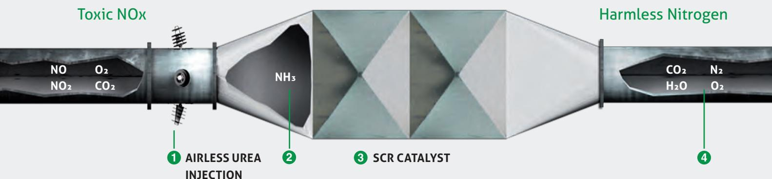
The Digital Airless Multipoint SCR process from toxic NOx to harmless nitrogen
